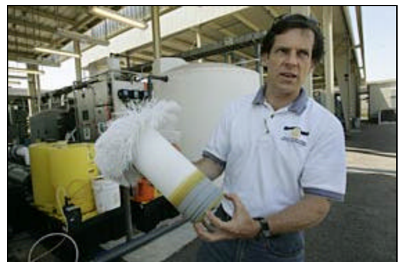
JOHN GIBBINS / Union-Tribune San Diego city water engineer Bill Pearce displayed a sample of one of the filters used in the process of turning wastewater into drinking water.
